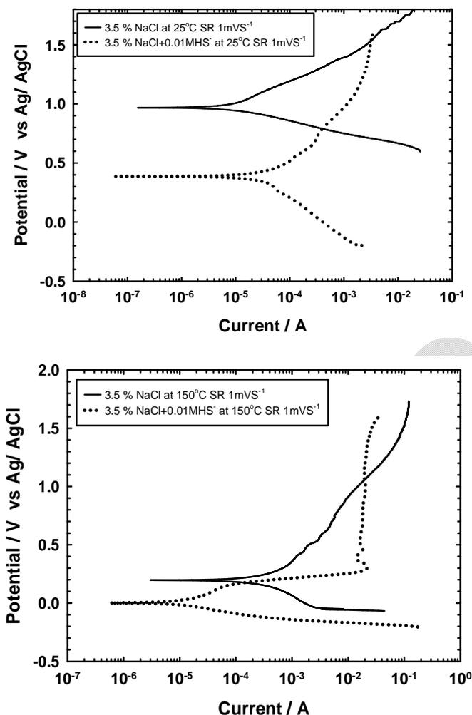
**Figure 3 (a, b):** Effect of sulfide ions on current-potential relation for the porous graphite electrode at a voltage scanning rate of  $1 \text{ mVs}^{-1}$  in 3.5% NaCl only and 3.5% NaCl +0.01 M  $\text{HS}^-$  at (A)  $25^\circ \text{C}$  (B)  $150^\circ \text{C}$ .
