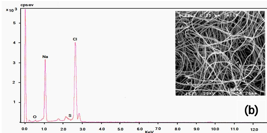
**Figure 7 (a, b):** (a) SEM and EDS of powder of evaporated used electrolyte containing  $0.01\text{M HS}^-$  at a potential of  $0.8\text{ V(Ag/AgCl)}$ , which was polarized by porous graphite electrode for 3 h at  $150^\circ\text{C}$ . (b) SEM and EDS of fibers of porous graphite electrode after it was polarized in a solution containing  $0.01\text{M HS}^-$  at a potential of  $0.8\text{ V(Ag/AgCl)}$  for 3 h at  $150^\circ\text{C}$ .
