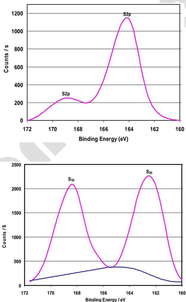
**Figure 5 (a, b):** XPS spectrum of the residual powder of an evaporated used electrolyte by rotary vapor device, the electrolyte is subjected for polarization at a potential of 0.8 V (Ag/AgCl) by using porous graphite electrode for 3 h, in presence of 3.5% NaCl + 0.01 M HS<sup>-</sup> at (a) 25° C and (b) 150° C.
