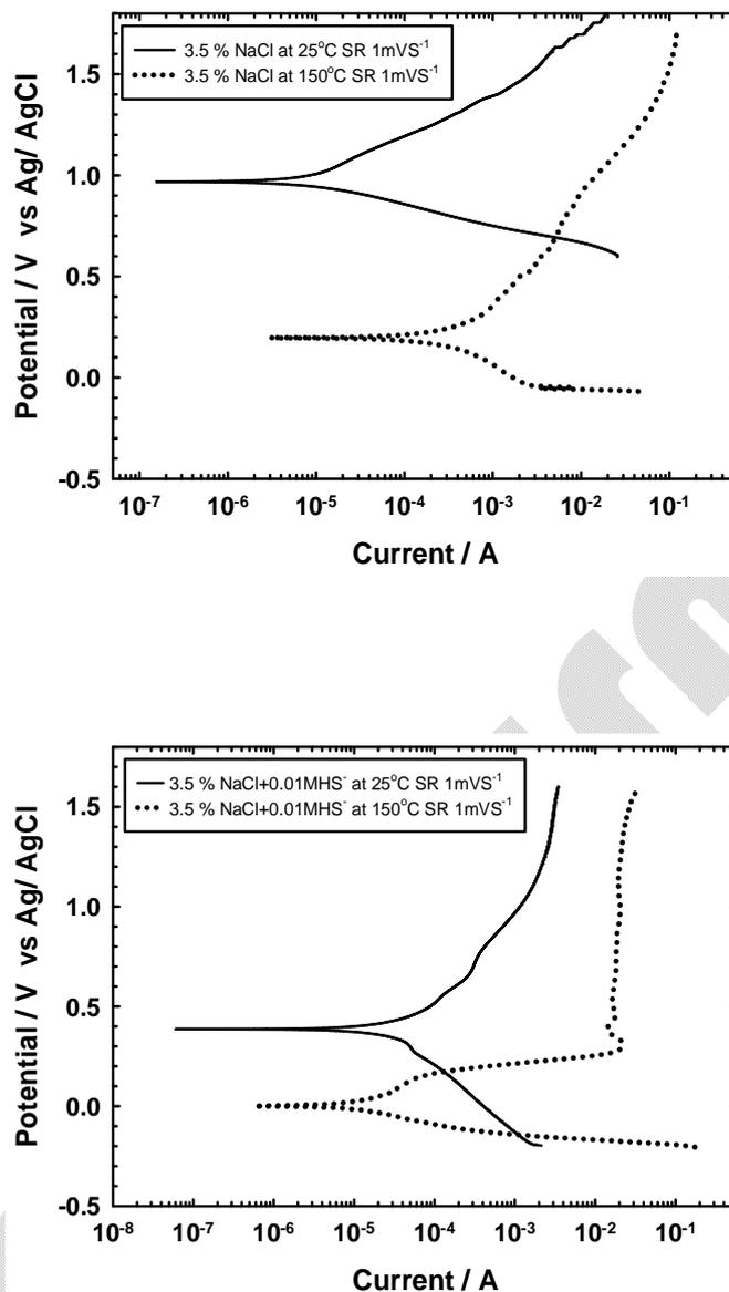
**Figure 2 (a, b):** Effect of temperature on current-potential relation of the porous graphite electrode at a voltage scanning rate of  $1 \text{ mVs}^{-1}$  in (a) 3.5% NaCl only and (b) 3.5% NaCl + 0.01 M  $\text{HS}^-$  at  $25^\circ \text{C}$  and  $150^\circ \text{C}$ .
