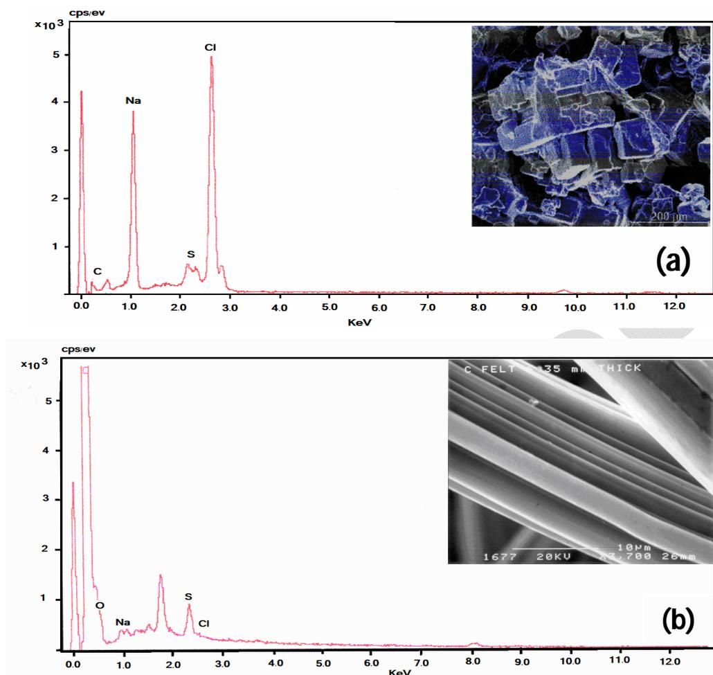
**Figure 6 (a, b):** (a) SEM and EDS of powder of evaporated used electrolyte containing 0.01M  $\text{HS}^-$  at a potential of 0.8 V(Ag/AgCl), which was polarized by porous graphite electrode for 3 h at 25° C. (b) SEM and EDS of fibers of porous graphite electrode after it was polarized in a solution containing 0.01M  $\text{HS}^-$  at a potential of 0.8 V(Ag/AgCl) for 3 h at 25° C.
