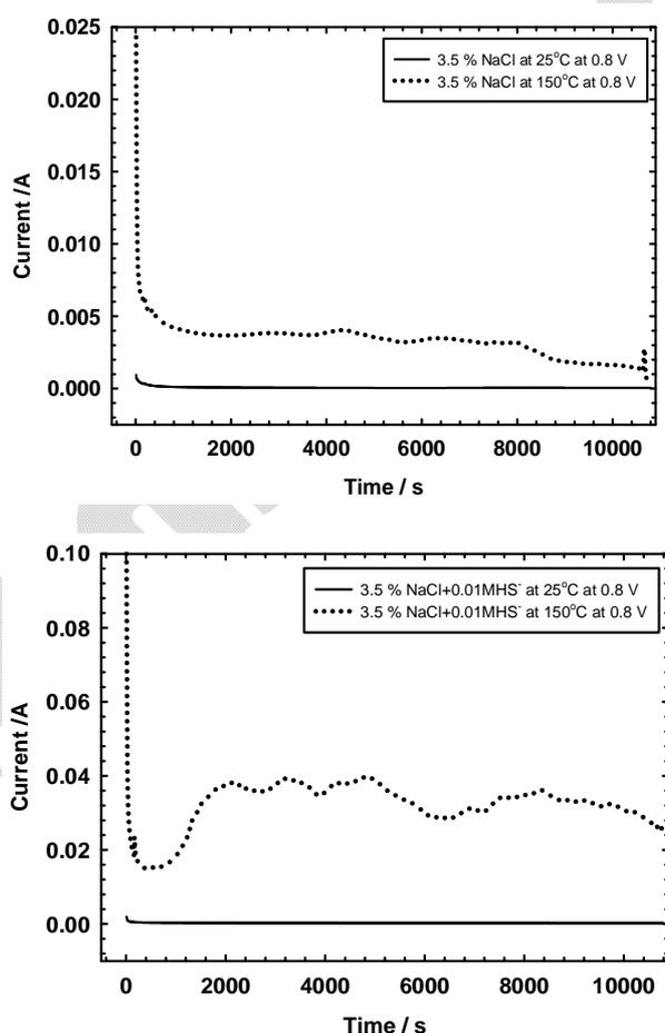
**Figure 4 (a, b):** Current transients supported by the porous graphite electrode at a potential of 0.8 V (Ag/AgCl) in (a) 3.5% NaCl at 25° C and 150° C, and (b) 3.5% NaCl+0.01 M HS<sup>-</sup> at 25° C and 150° C.
