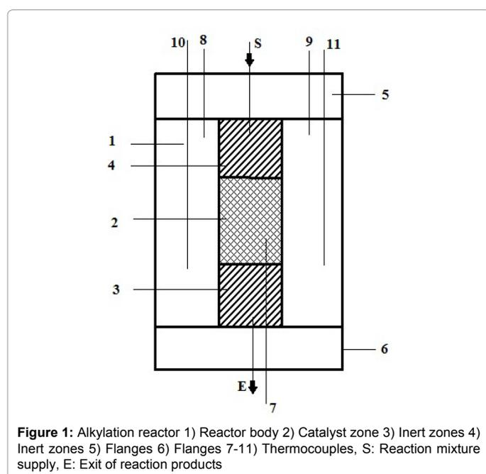
Figure 1: Alkylation reactor 1) Reactor body 2) Catalyst zone 3) Inert zones 4) Inert zones 5) Flanges 6) Flanges 7-11) Thermocouples, S: Reaction mixture supply, E: Exit of reaction products
