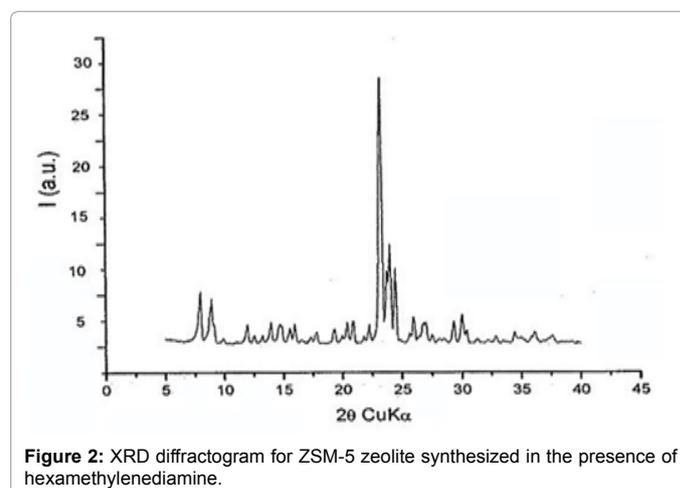
Figure 2: XRD diffractogram for ZSM-5 zeolite synthesized in the presence of hexamethylenediamine.
