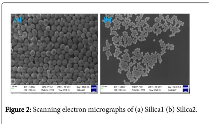
Silica samples were prepared using two different TEOS concentration of 3 M and 0.8 M while ammonia and water concentrations are fixed at 1.4 M and 6 M respectively.
