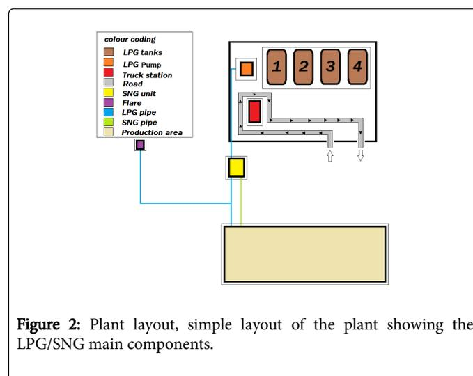
**Figure 2:** Plant layout, simple layout of the plant showing the LPG/SNG main components.
